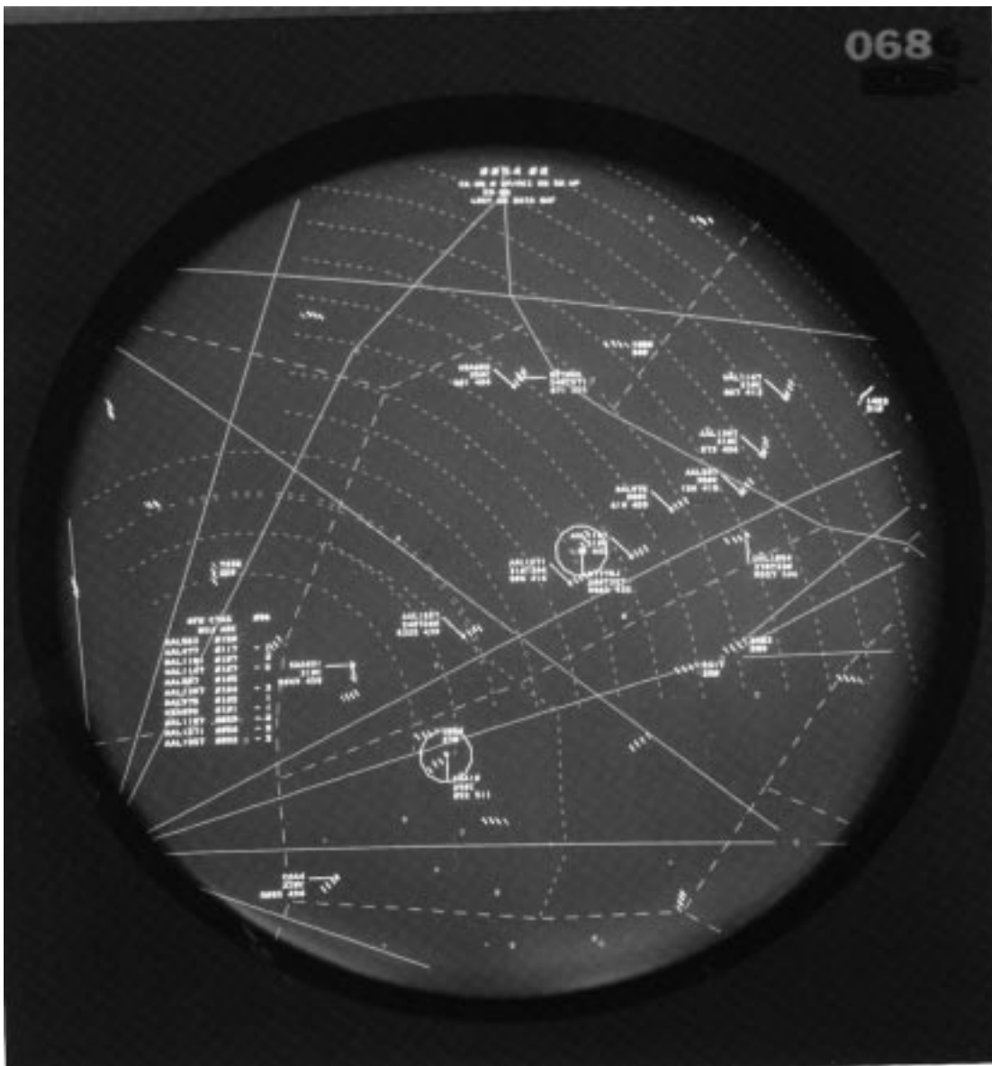
Figure 5. Controller PVD with TMA advisories displayed 1st USA/Europe Air Traffic Management Research & Development Seminar Saclay, France, June 17 - 19, 1997
