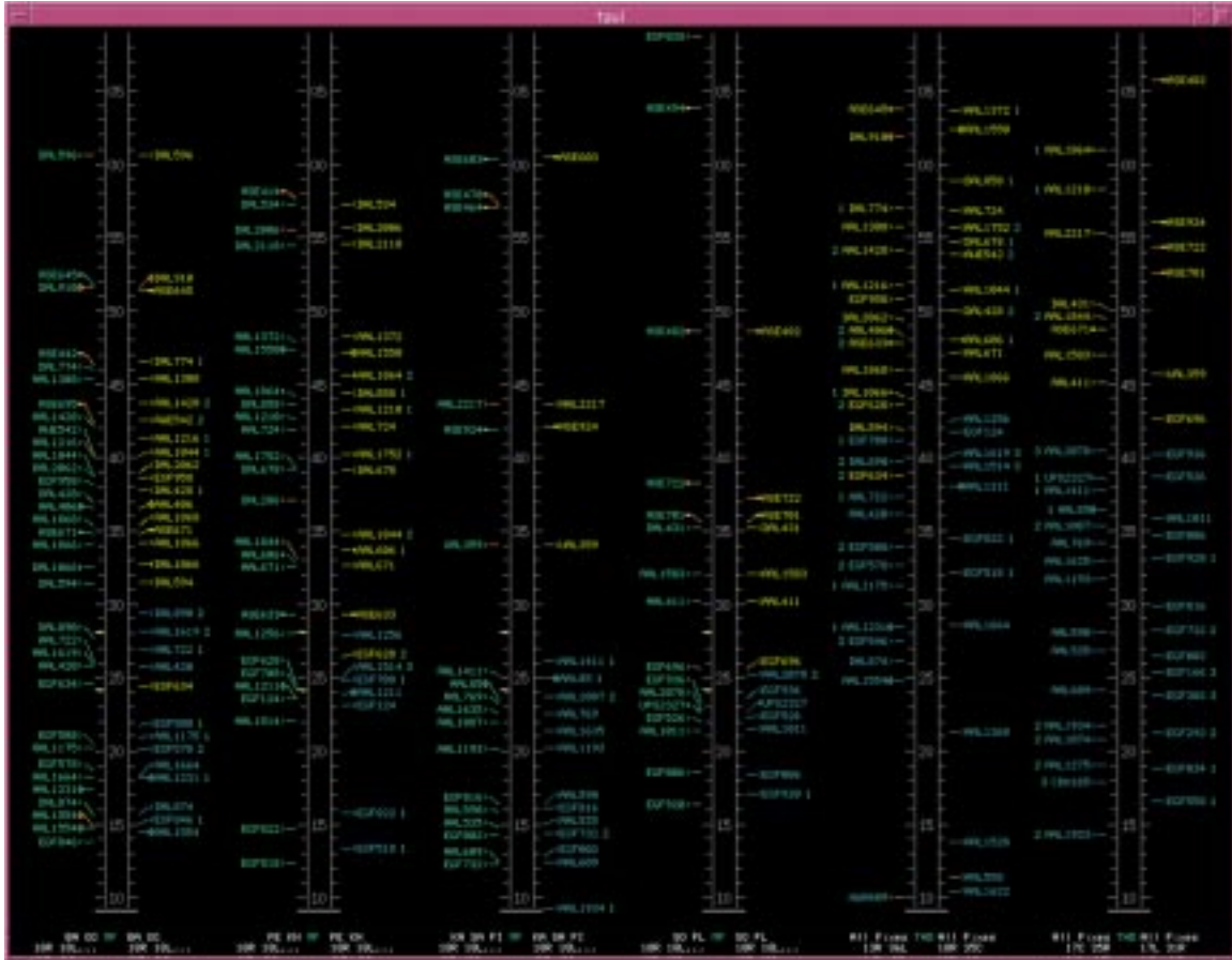
Figure A.1. TGUI timelines. This figure shows the basic TMA display of timeline information. Each timeline is referenced to meter fixes or runway threshold.
