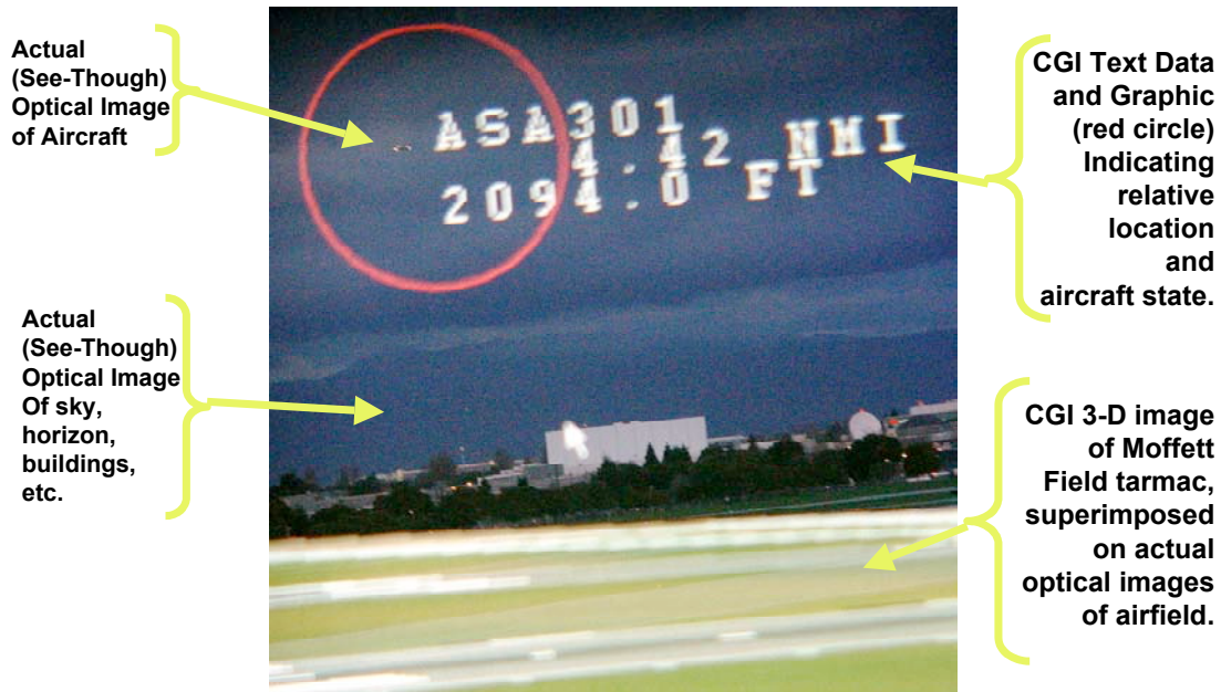
Figure 8. Photo was taken through an ARTT 2.0 'see-through' display at Moffett ATC Tower. The lights and optical image of the aircraft (ASA301) are framed by the CGI red circle and labeled by the adjacent data block.
