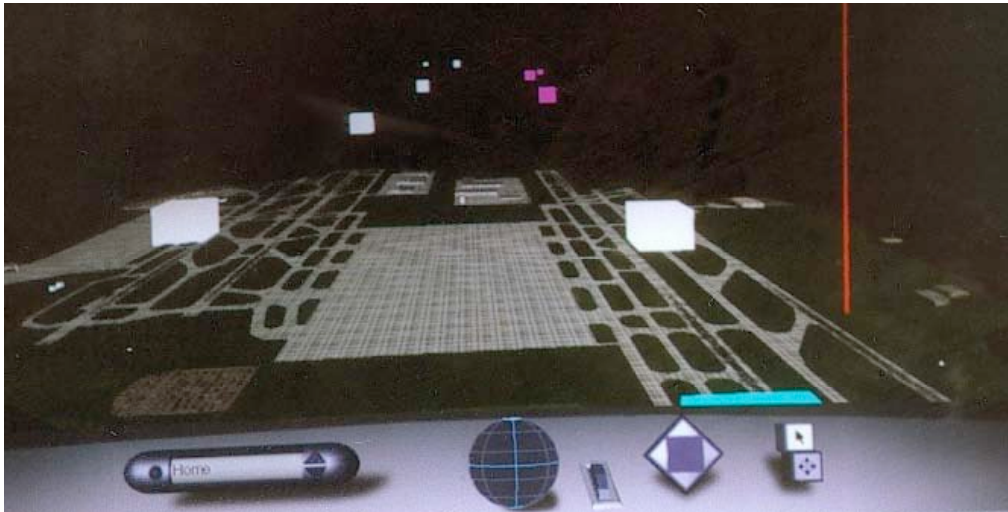
Figure 1. Situation Awareness Virtual Environment (SAVE) used realtime ATC radar to represent aircraft as ‘cubes’ viewed over a 3-D display of the airport.
