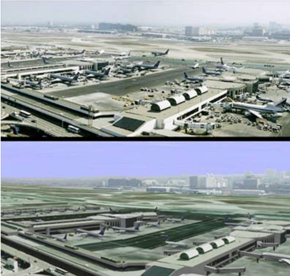
Moving vehicles such as aircraft and service trucks were modeled in 3D, and moved about the airport scene under the control of "pseudo-pilots" who occupied the downstairs stations in FutureFlight. Pseudo-pilots controlled pushback time, taxi route, speed, take-off and landing in coordination with ATC in the virtual tower. Engineers used daytime conditions for the scene, although other times of day are possible. They modeled both clear day visibility and fog.
