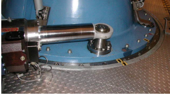
Figure 6: Yaw actuator with existing rod end.
