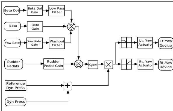
**Figure 8 Modified Yaw Control System**
