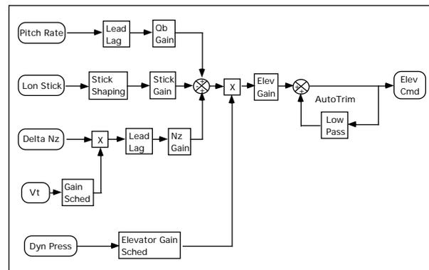
**Figure 2 Pitch Command Generator**
