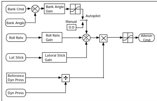
**Figure 3 Roll Command Generator**
