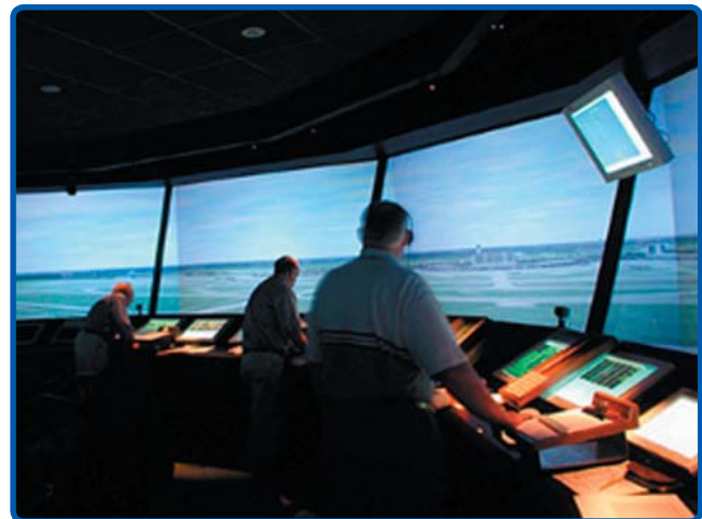
View from the FFC control tower. Because of HLA bridging technology, multiple simulators can participate in the same scenario in real-time.
