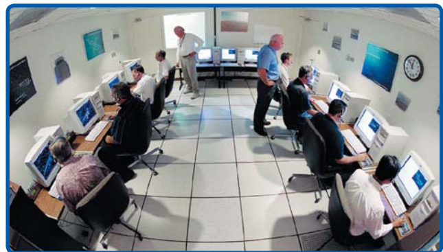
CVSRF's ATC simulator can operate independently or linked with the flight simulators.
