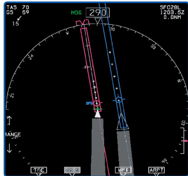
A screenshot of the NAV display during a CSPA. The RIA is shown on the left, and the CTOL is shown on the right.
