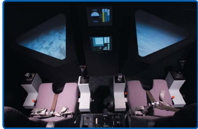
Interior of a VMS cab, configured for the Lunar Lander Module simulation. The lunar surface is visible through the Apollo-style triangular windows.
