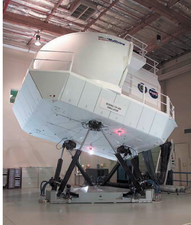
The NASA Ames B747 Level D flight simulator is shown above. The motion actuator drive equations were tuned to use the full range of actuator extension.
