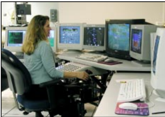
The Development Work Station gives researchers tools for developing and evaluating aircraft models in a simulation environment; these models can then be imported directly into the VMS system.
