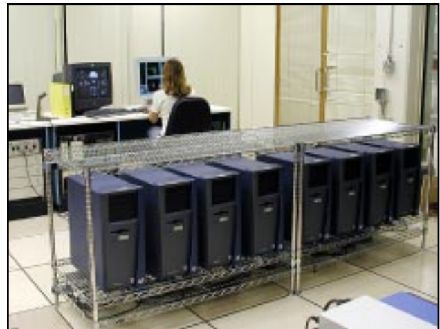
Real-time cockpit avionics displays at SimLab are now generated on PC-based graphics engines running an open Operating System and Open Graphics Libraries.
