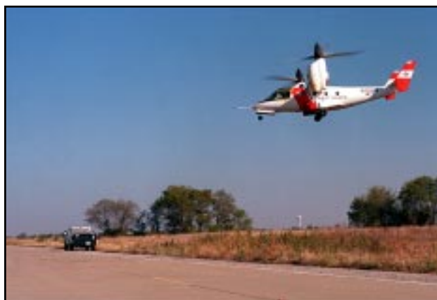
The XV-15 tiltrotor aircraft conducting noise abatement profile testing from profiles generated at the VMS.
