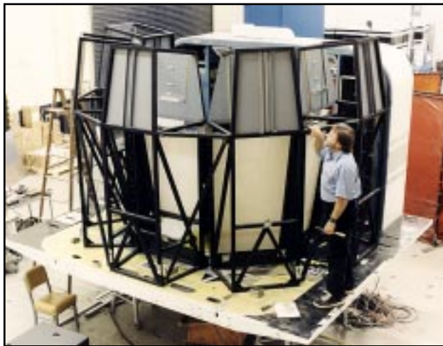
The newly rebuilt N-cab undergoing modification to enhance the field of view with five projectors displaying the out-the-window view for the pilot.
