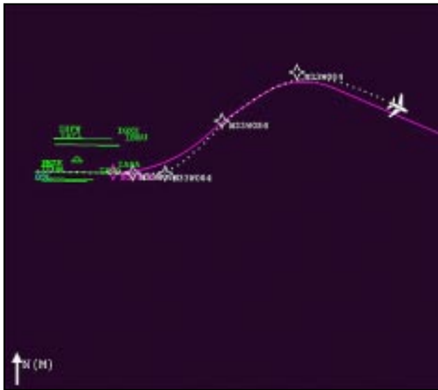
A map showing the ground track of the aircraft with respect to the FMS computed track (solid line) part way through a departure at unrestricted airspeed.
