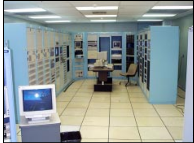
Centralized video switching and processing resources provide the VMS with a highly flexible and efficient environment to support multiple simulations.
