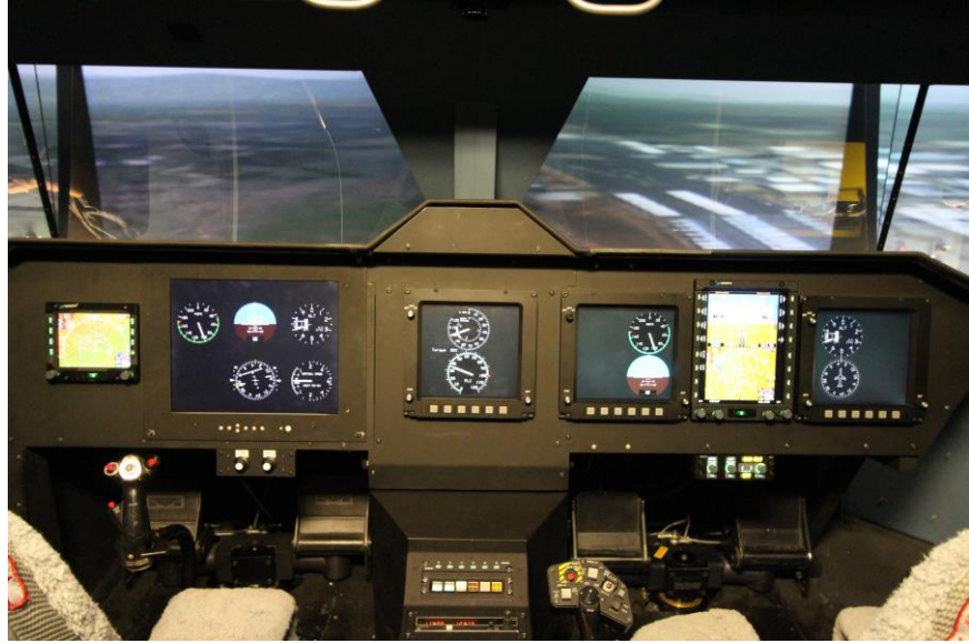
Fig. 2 Advanced Rotorcraft Two-Seat Cab, Flight Hardware and Controllers
