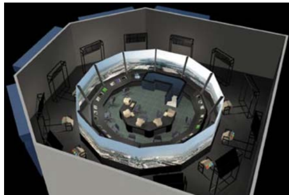
Figures 2a and 2b. FutureFlight Central. Tower scene from FutureFlight Central with the screen and projector layout.
