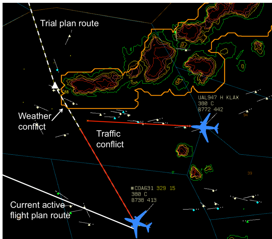
Figure 6: Example of trial plan with weather and traffic conflicts that would prevent DWR from suggesting this route.
