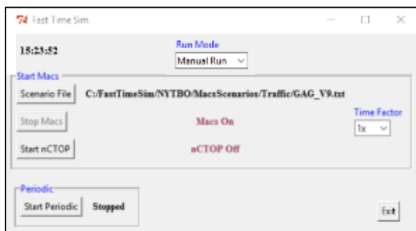
Figure 3. A Graphical User Interface (GUI) to set up communication between MACS and nCTOP and set MACS parameters.
