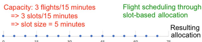
Fig. 3. Example of flight scheduling through slot-based allocation: 3 flights are evenly spaced within each 15-minutes time-interval.
