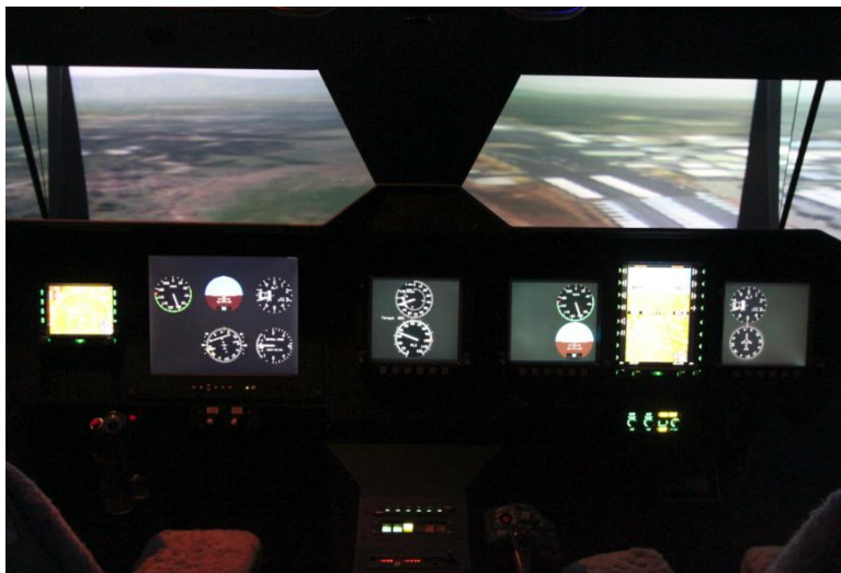
Figure 2. Advanced rotorcraft cab interior for full-mission scenarios.
