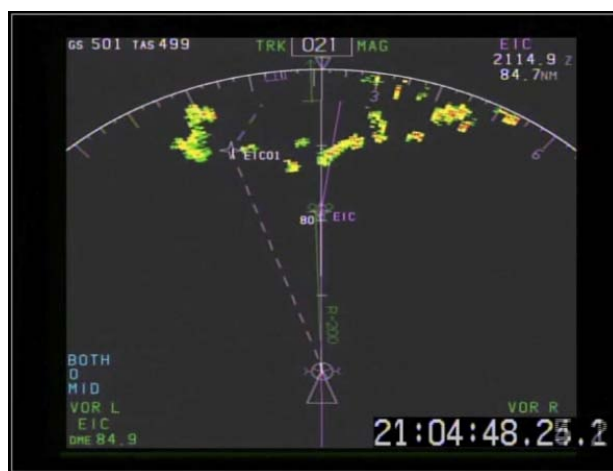
Figure 6. 747-400 Navigation Display Showing Route Loaded but not Executed
