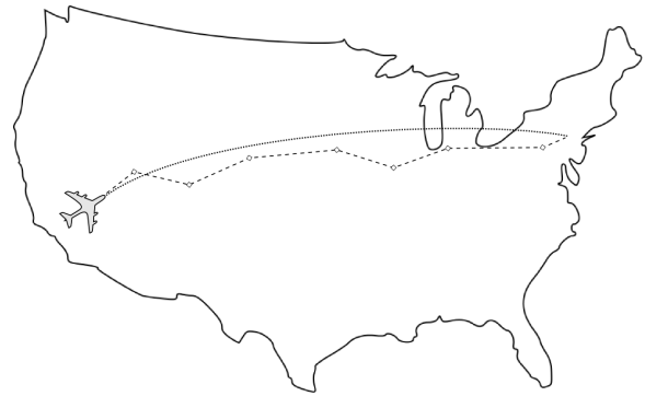
Figure 7: The simulation is capable of allowing self-separating aircraft to fly direct routes (dotted) instead of structured routes (dashed).
