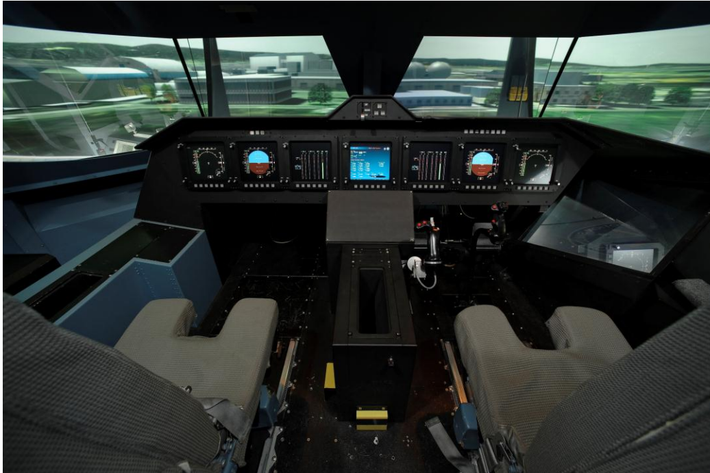
Figure 3. Example Two-Seat Cab with Tilt-Rotor Controls and Displays
