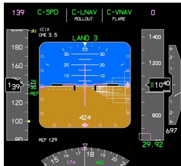
Figure 4: Primary Flight Display
