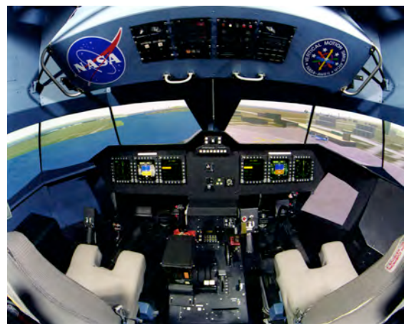
Figure 2. Exterior and interior of Transport Cab (TCAB) with eight out-the-window visual displays
