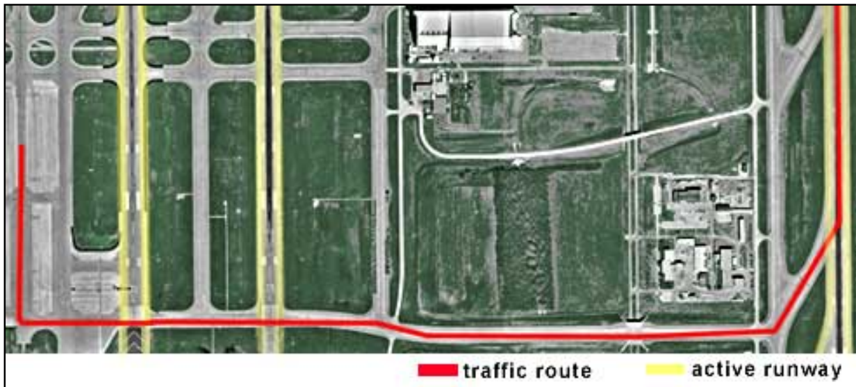
Figure 4: The aerial photograph above shows a typical eastside DFW south flow arriving traffic route with runway crossings. (Only a portion of the eastside is depicted.)
