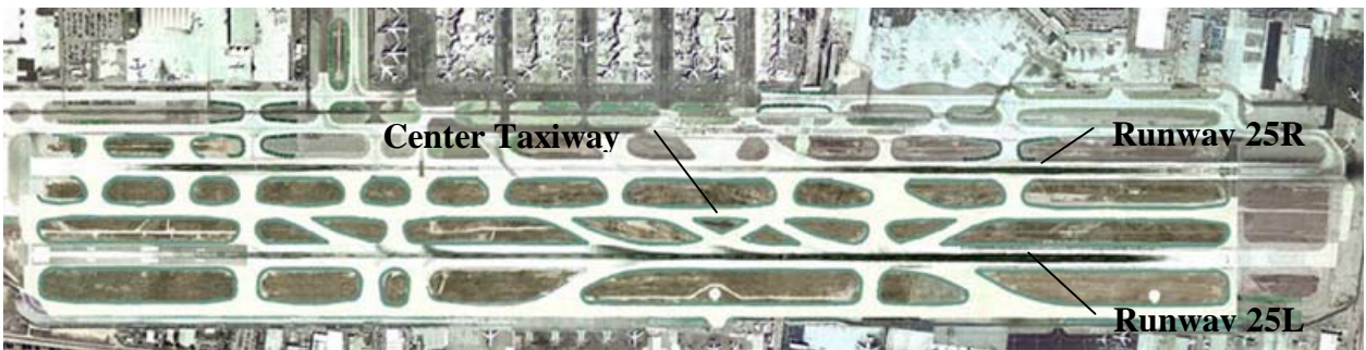
Figure 2: Center taxiway Concept, South Complex at LAX
