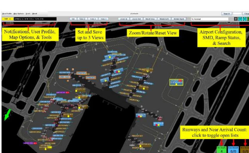
Ramp Traffic Console (RTC) and Ramp Manager Traffic Console (RMTc)
